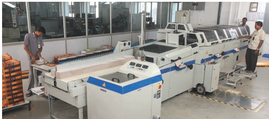
Kolbus DA 280 Case maker - 100 cases / min. India's first installation as on 2011 Sep
