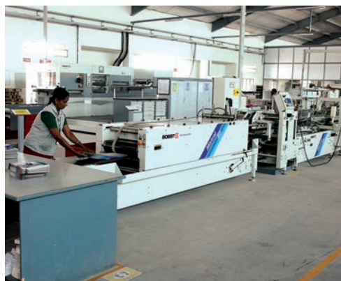
Bobst Mistral 80 - Box Pasting 400 meter / minute
