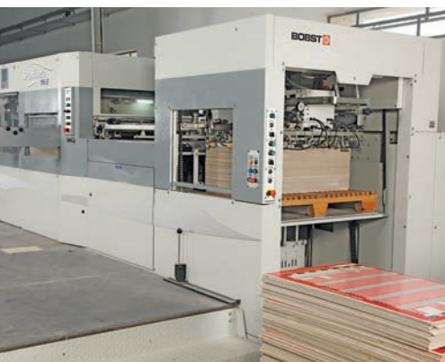
Spanthra 106LE Die Cutting - 9000 Sheets / Hour with auto register
