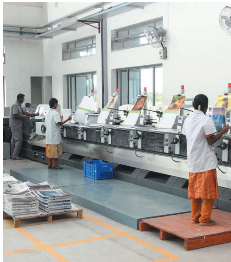
Heidelberg ST 350 Saddle Stitcher line - 12,000 Books / Hour with Quality inspection feature
