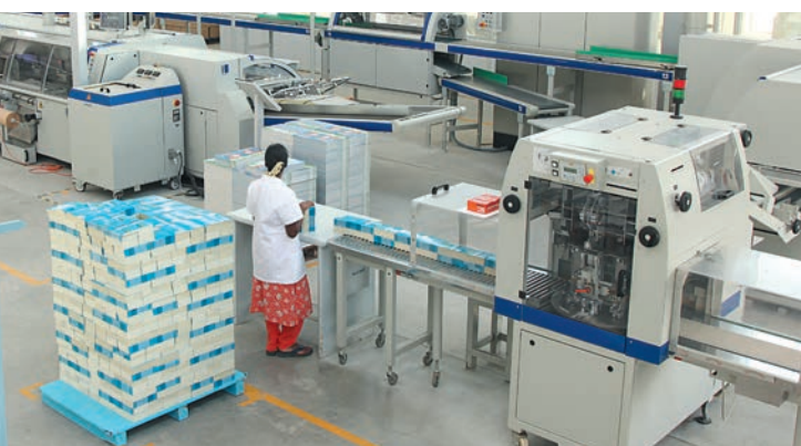
Kolbus KM 600-7000 Softcover Books/hour with Signal X camera
