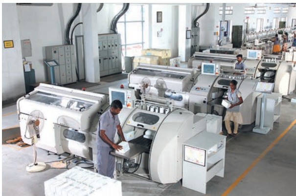
21 station gatherer connected to 3 nos of Aster 220C-39,600 Signatures / Hour - Machine with Signal X camera & Image reader Asia's First Installation as on 2009 Nov
